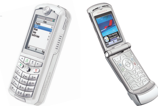
Both the Rokr (left) and Razzr (right) mobile phones incorporate Freescale Semiconductor's dual-core DSP56631 baseband processor and the quad-band MC13777 GPRS front-end ICs.
